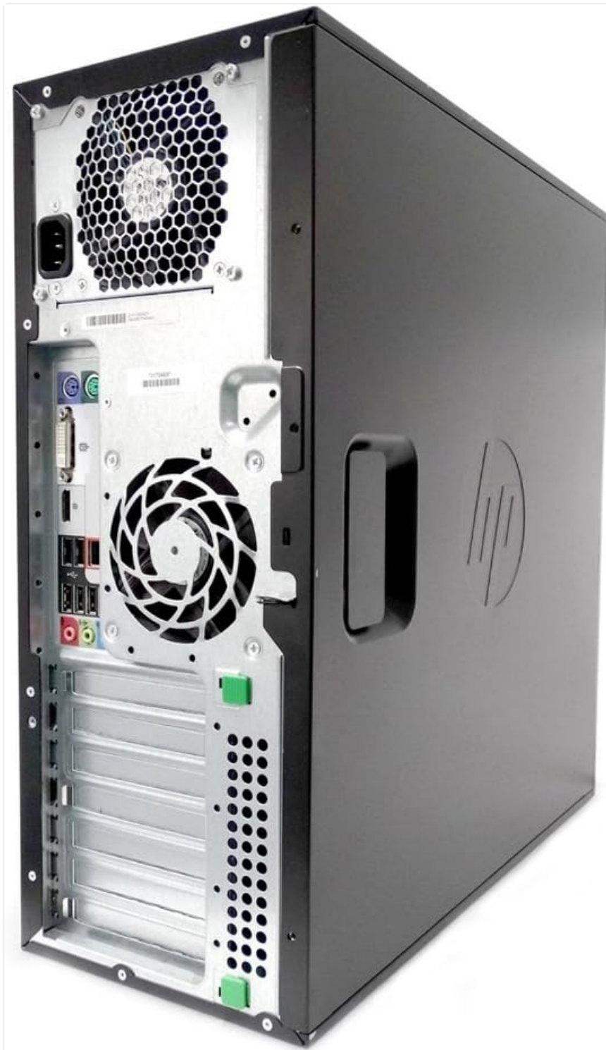
Figure 3.1: Rear view of the HP Z210 Workstation Tower, illustrating the various input/output ports for connecting peripherals and power.
