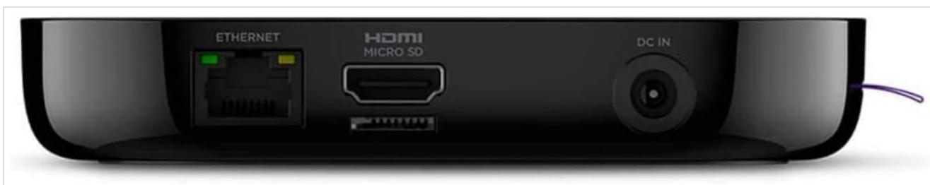
Figure 1: Rear ports of the Roku Ultra player. Connect the HDMI cable here.
