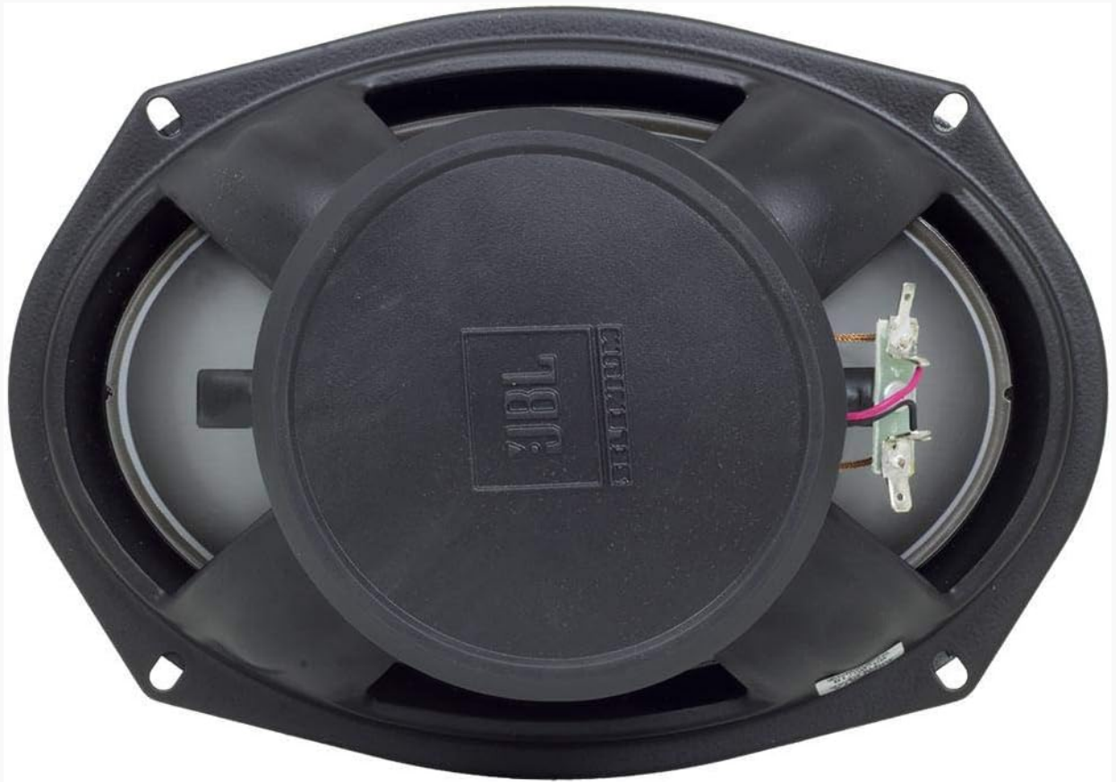
Image 3.2: Rear view of a JBL 69QD9TA speaker, highlighting the magnet structure and wiring terminals. Proper connection to these terminals is essential for speaker function.
