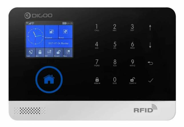
Figure 4.1: Front view of the Digoo DG-HOSA control panel, displaying the touchscreen interface, numeric keypad, and function buttons for system control.
