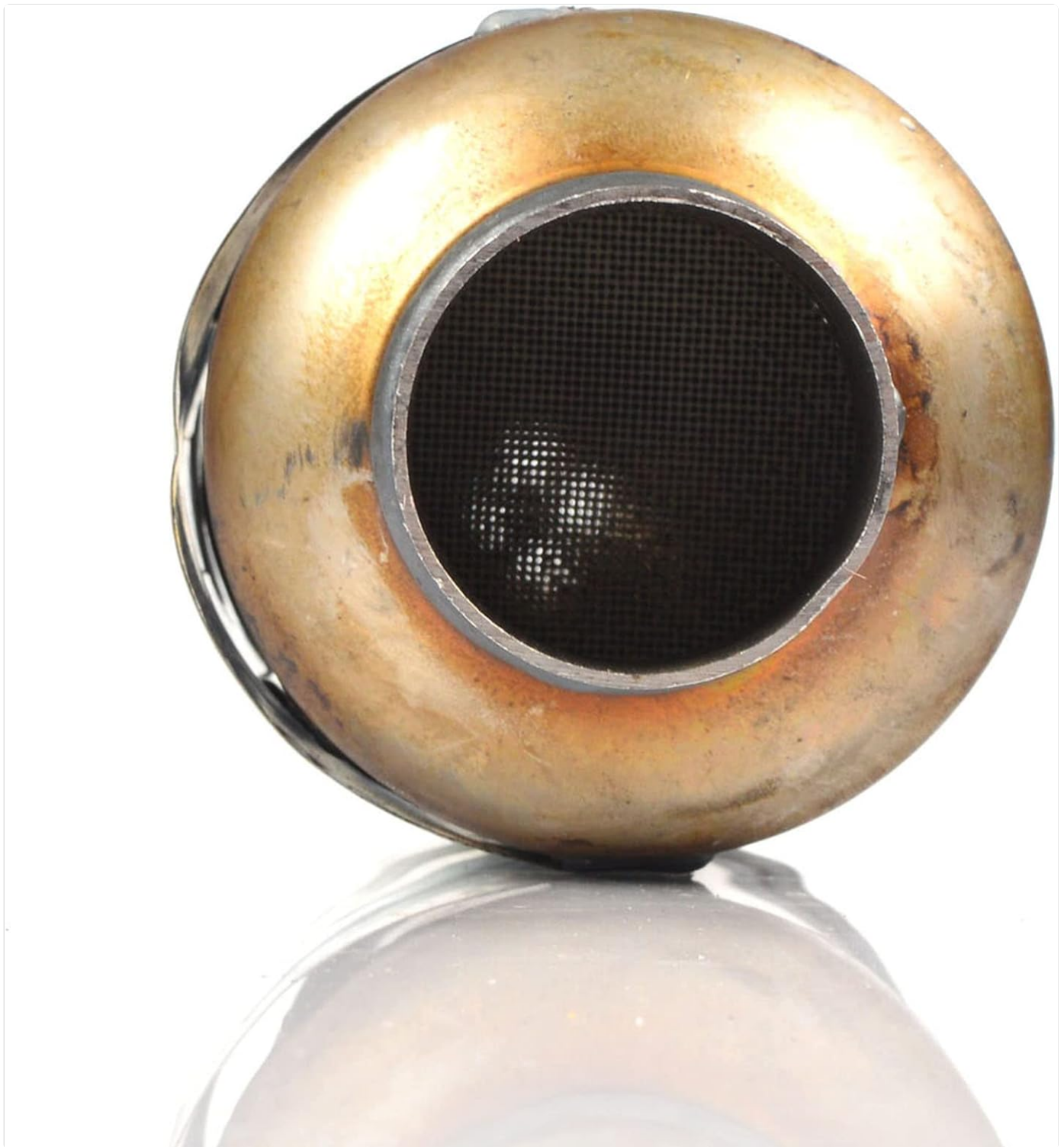
Image 6.1: End view of the catalytic converter, revealing the internal honeycomb structure where catalytic reactions occur.
