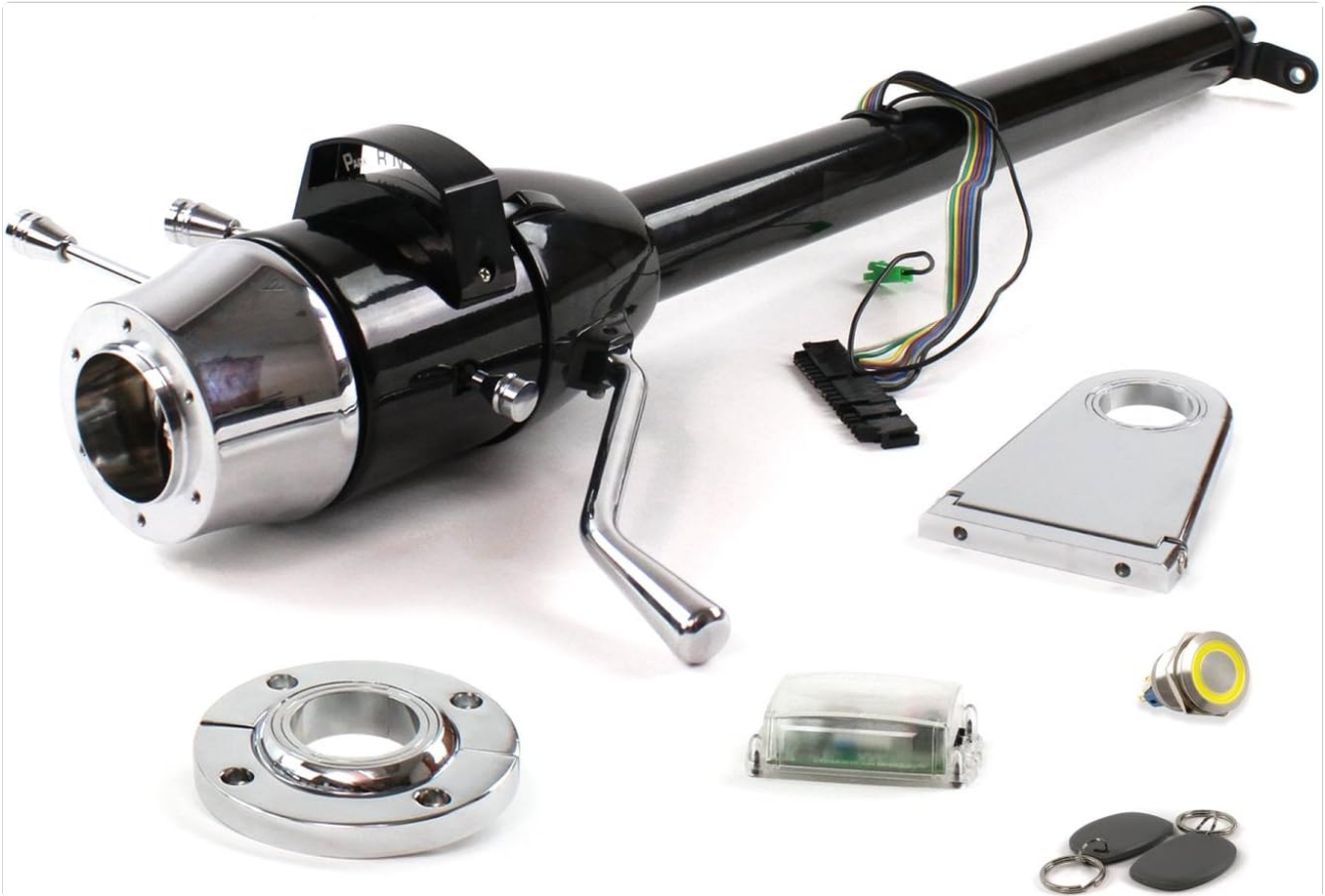
Figure 1: Overview of the Helix 706622 Column Shift and included components. This image displays the main black tilt steering column, a chrome floor mount bracket, a clear RFID module, a yellow-ringed push-button start switch, and two black RFID key fobs.
