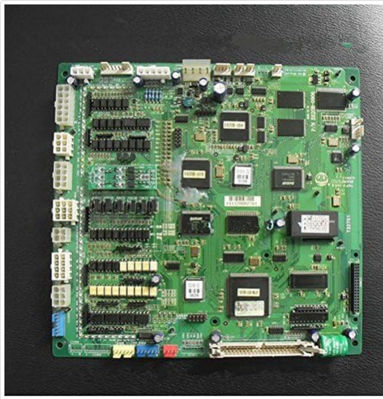
Figure 2.1: Top view of the GOWE Dahao Embroidery Machine Motherboard, showing various integrated circuits, connectors, and components. This image displays the overall layout and design of the main board.
