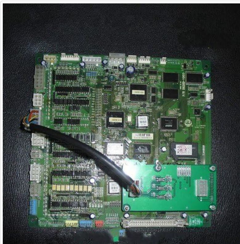
Figure 2.2: The GOWE Dahao Embroidery Machine Motherboard with a black data or power cable connected to one of its ports. This illustrates a typical connection point on the board.
