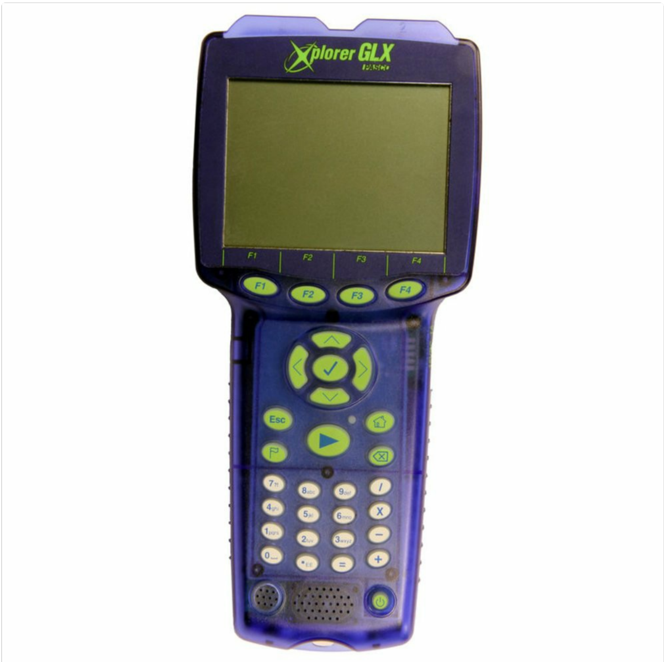
Figure 1: Front view of the PASCO PS-2002 Xplorer GLX Graphing Logger. This device features a large LCD screen for data display, function buttons (F1-F4) for quick access, a central navigation pad, a numeric keypad for data entry, and a power button at the bottom. The casing is a translucent blue with green accents on the primary control buttons.
