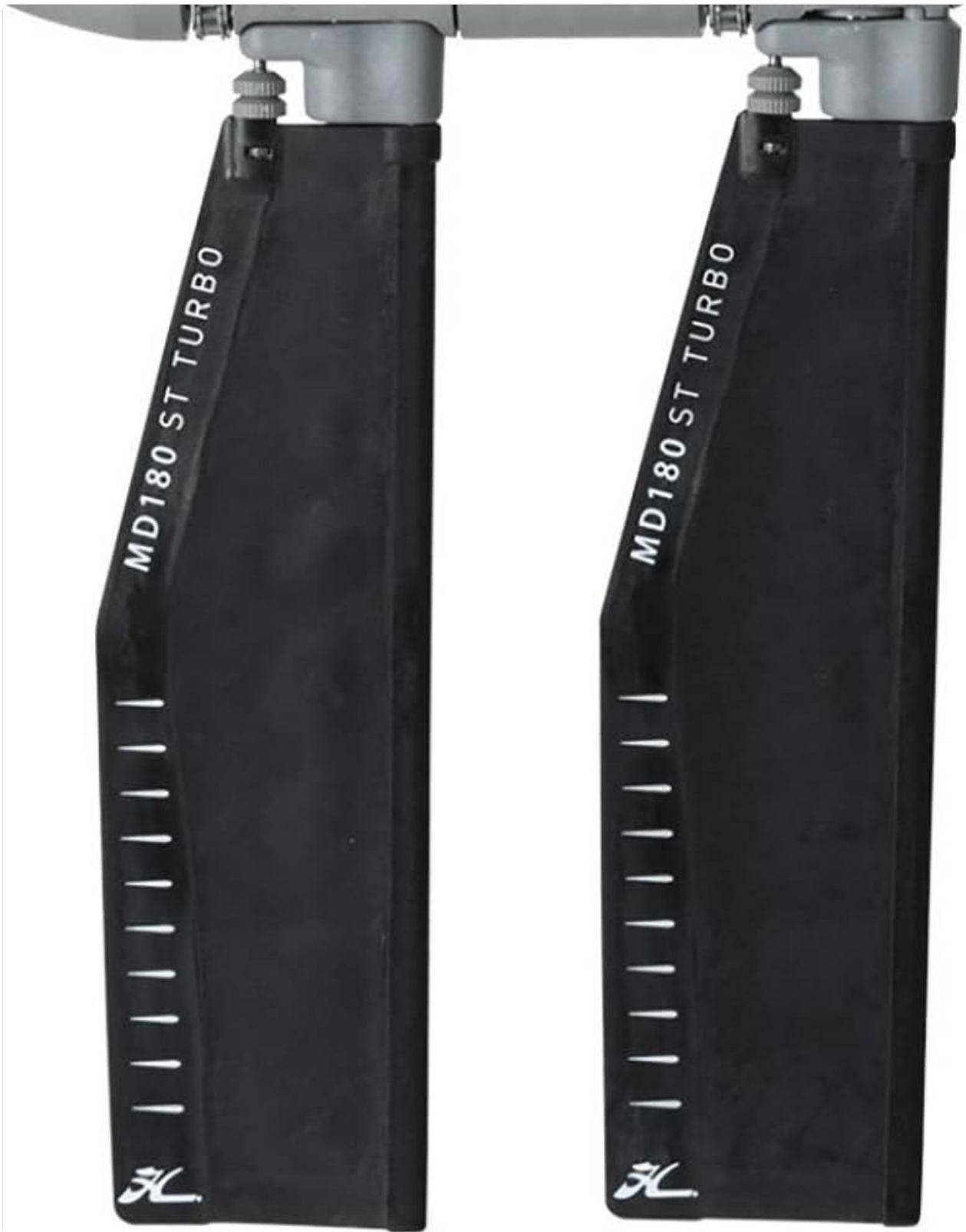
Image: A Hobie Mirage Drive unit with the new MD180 ST Turbo fins properly installed. The fins are securely attached to the drive's masts, ready for operation.
