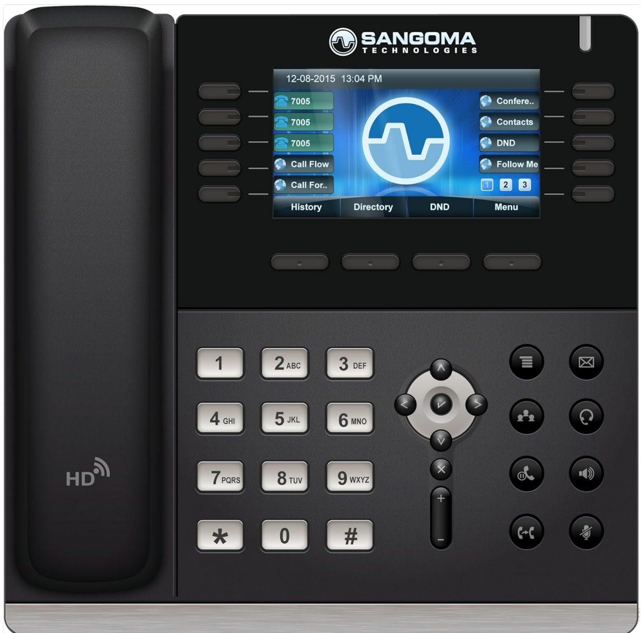
Figure 1: Sangoma s705 VoIP Phone Front View. This image displays the front of the Sangoma s705 phone, highlighting its large display screen, numeric keypad, navigation cluster, and various function buttons. The handset is visible on the left side. The display shows "SANGOMA TECHNOLOGIES" logo, date and time (12-08-2015 13:04 PM), active lines (7005), and menu options like Conference, Contacts, DND, Follow Me, History, Directory, and Menu. The keypad includes standard numbers, asterisk, hash, and volume controls.
