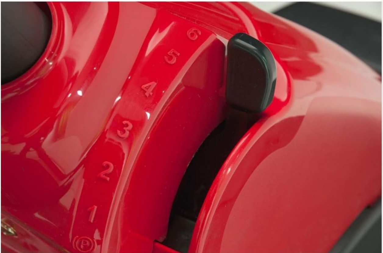
Figure 2: The gear shift lever for selecting one of the 6 available speeds or Park (P).
