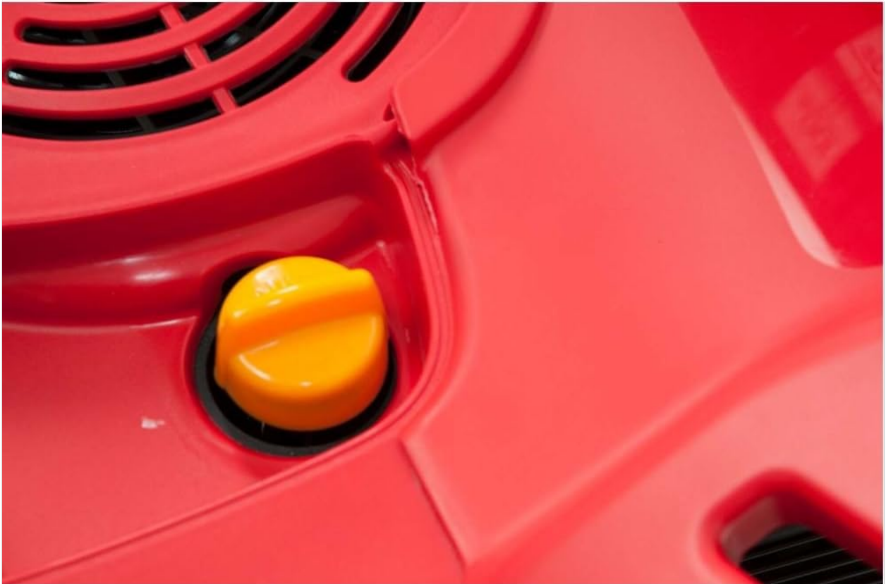
Figure 3: The yellow cap indicates the engine oil filler and dipstick location for checking and adding oil.
