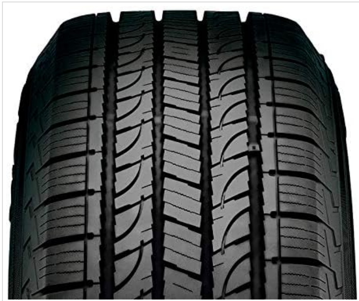
Close-up of the tire's tread blocks, illustrating the detailed siping for enhanced grip.
