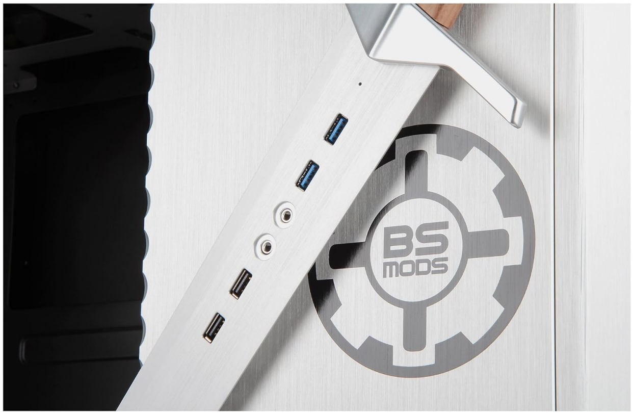
Figure 2: Detailed view of the sword-designed I/O panel, highlighting the USB ports and power button.
