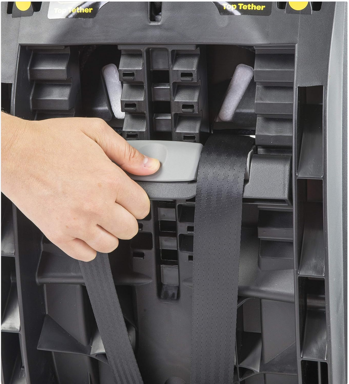
Image 4.1: A hand demonstrating the adjustment mechanism for a car seat strap, likely part of the ISOFIX or top tether installation process, located on the underside of the seat base.
