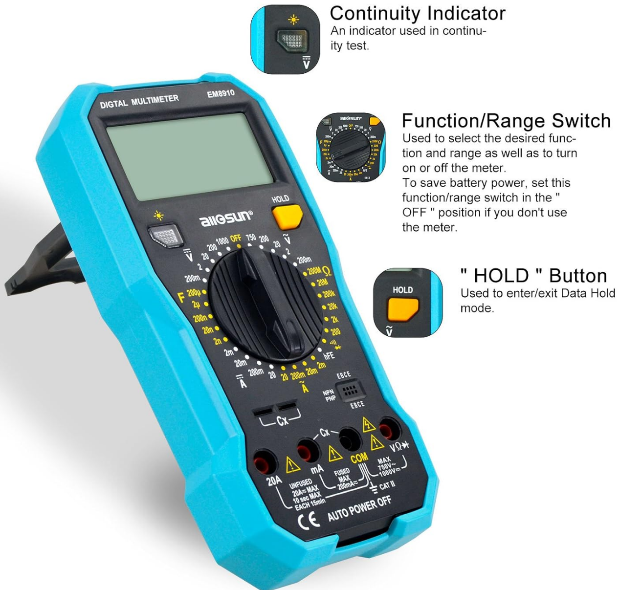
Figure 3.3: Detailed view of the Continuity Indicator, Function/Range Switch, and HOLD Button.
