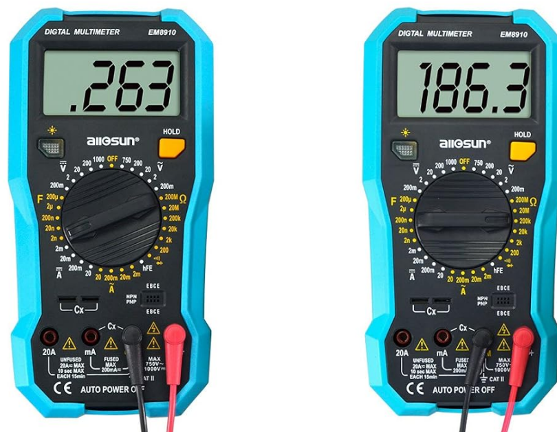
Figure 5.1: Measuring Resistance and Capacitance with the EM8910 Multimeter.
