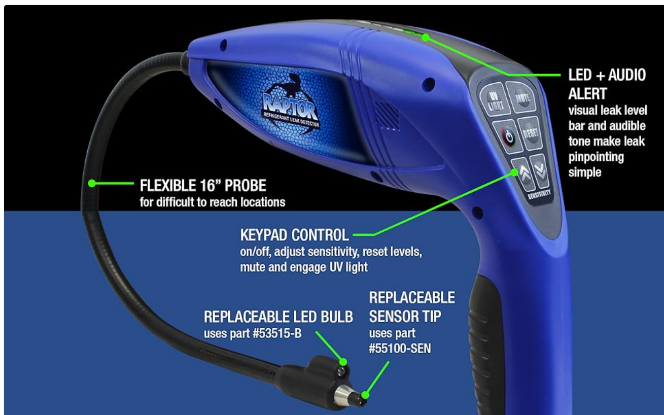
Image: An annotated diagram of the Mastercool 56200, clearly indicating the location of the replaceable sensor tip (part #55100-SEN) and the replaceable UV LED bulb (part #53515-B) on the probe, along with the LED and audio alert system and keypad controls.
