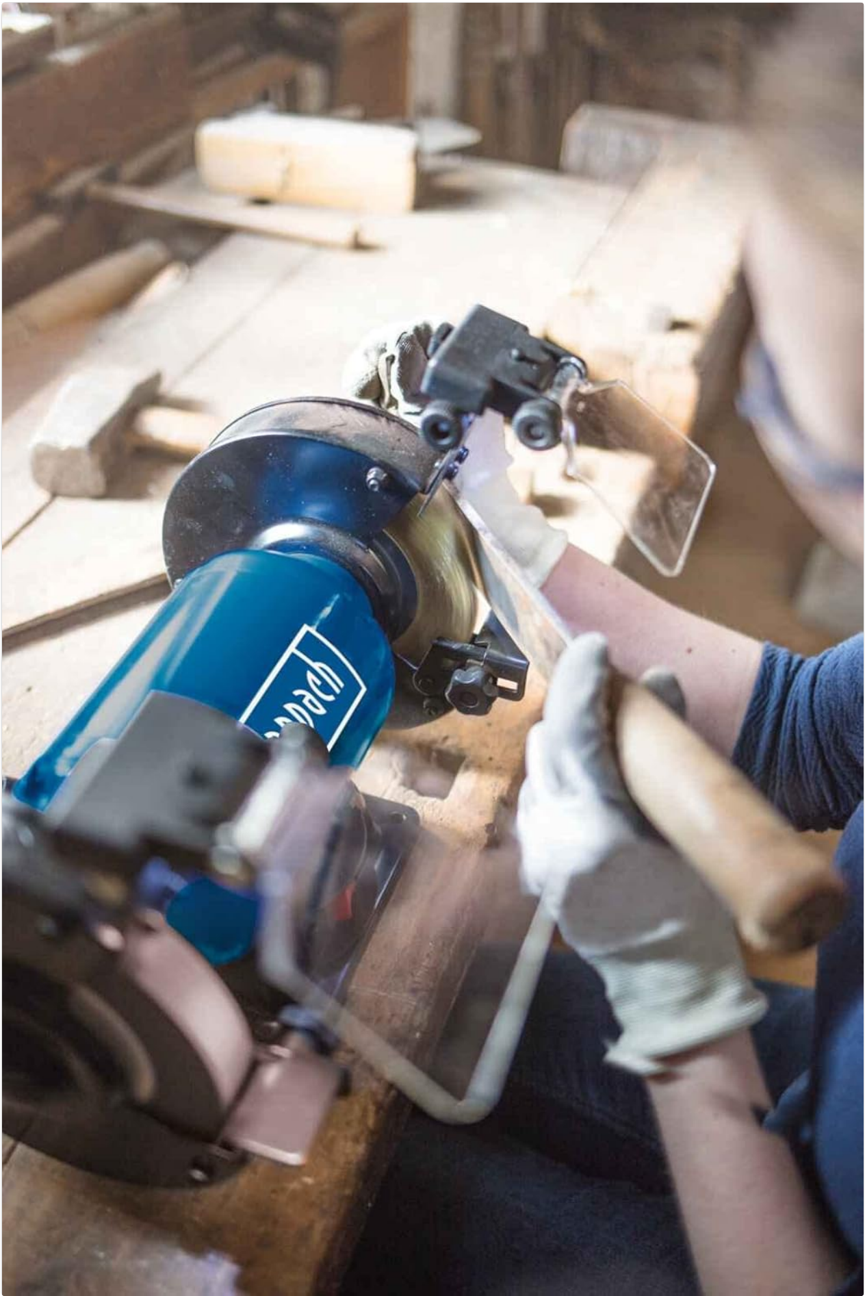
Figure 5.5: A close-up view illustrating the precise contact between the chisel and the grinding wheel during sharpening.
