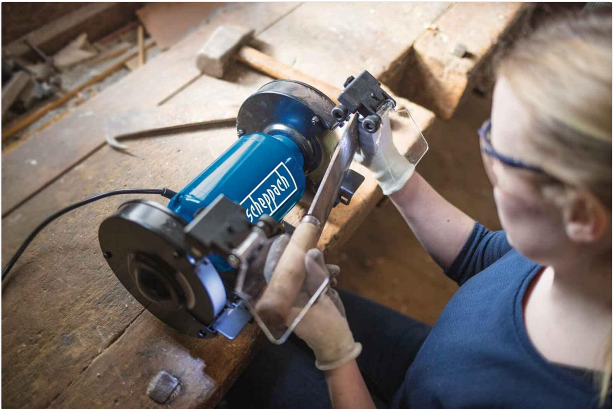
Figure 5.4: A user sharpening a woodworking chisel, demonstrating the versatility of the grinder for various tools.
