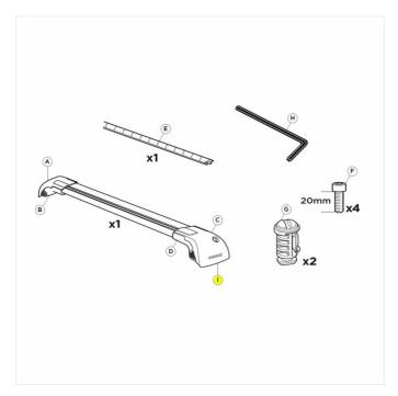
Image: An exploded diagram illustrating various components of a Thule roof bar system. Key parts include the roof bar (A), end caps (B, D), rubber strip (E), and the screw (F). The screw (F) is depicted with dimensions 20mm and a quantity of x4, indicating its role in securing multiple points of the roof bar assembly. An Allen key (H) is also shown, suggesting the tool required for tightening.
