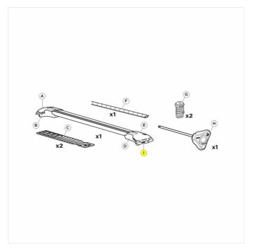
Image: Another exploded diagram of Thule roof bar components. This illustration features a different type of fastener (G) and a torque wrench (H) with a specified setting of 2Nm. While this diagram shows a different fastener, it emphasizes the importance of precise tightening for secure installation within the Thule system.
