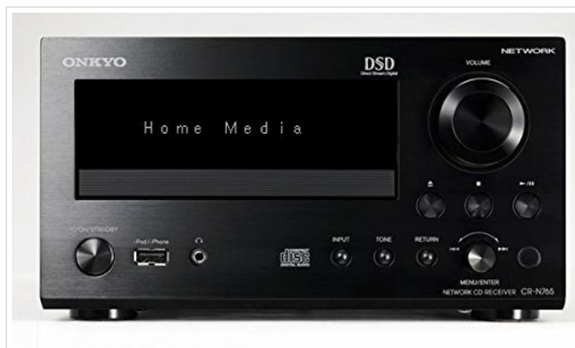
Figure 3: Network Media Display. This image shows the front of the Onkyo CR-N765, with the display indicating 'Home Media', signifying that the unit is ready to access content from your local network.
