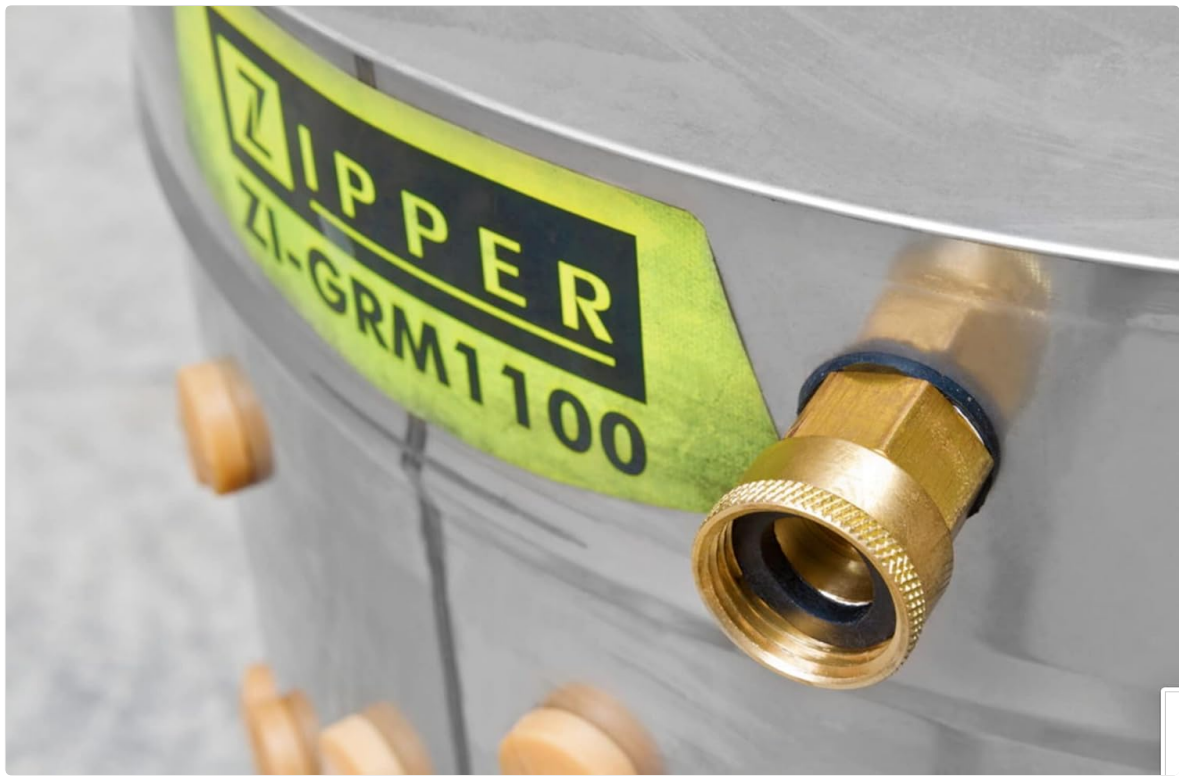
Figure 3.2: Close-up view of the water inlet connection. This brass fitting allows for a hose to be attached, providing a continuous water supply to rinse feathers during the plucking process, enhancing efficiency and hygiene.
