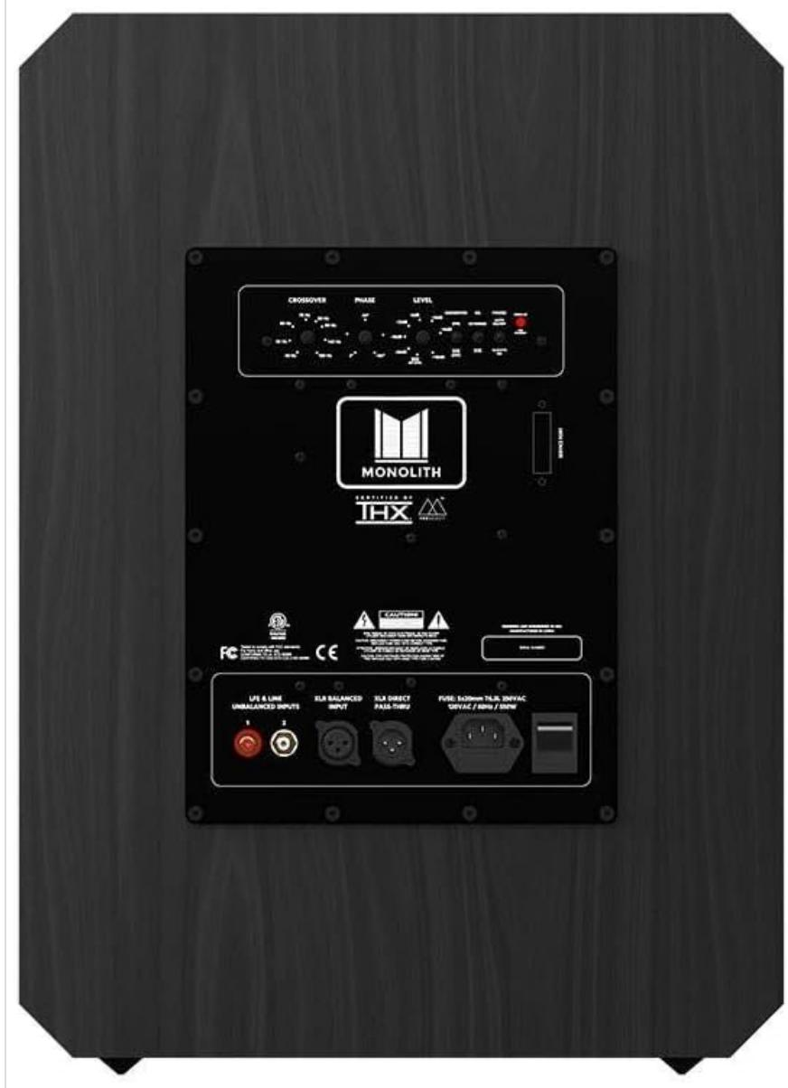
The rear panel houses all the necessary connections and controls for the subwoofer. This includes inputs for audio signals, power input, and various adjustment knobs for fine-tuning the sound. Key controls typically include Crossover, Phase, and Level (volume).
