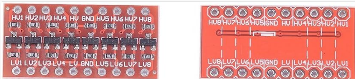
Image 4.1: Detailed view of the CYT1082 module, highlighting the HV, LV, and GND pins, along with the 8 data channels (HU1-HU8 and LU1-LU8).
