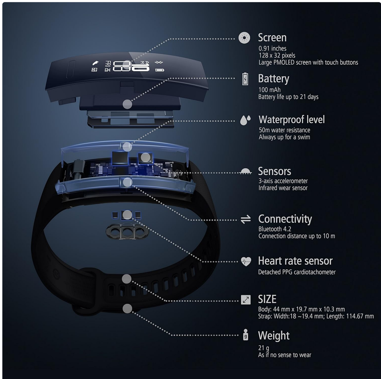
Figure 5: Exploded view of the Huawei Band 2, detailing internal components and key specifications such as screen, battery, waterproof level, sensors, connectivity, heart rate sensor, size, and weight.
