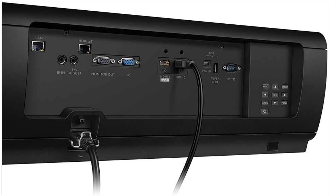
Figure 3: Rear panel of the BenQ LK970 4K Laser Projector, displaying various input and output ports including HDMI, LAN, HDBaseT, and USB.
