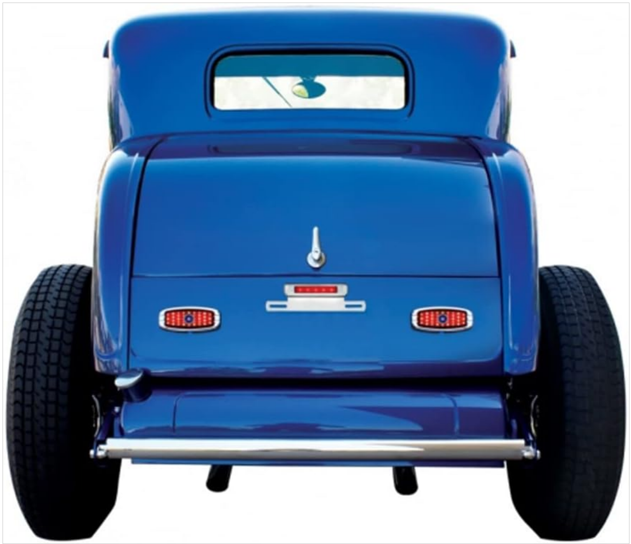
Figure 2: The S2007LED unit mounted on the rear of a vehicle, demonstrating its placement above the license plate.
