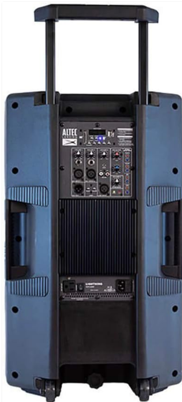
Figure 2: Rear panel of the ALP-L2200PK, illustrating the various input and output connections.
