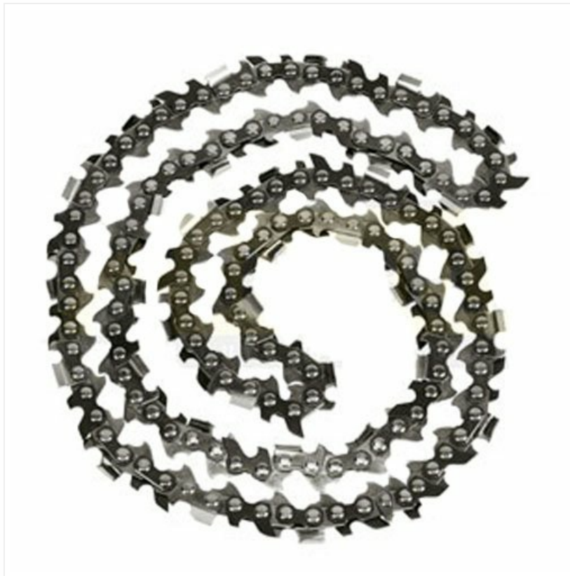
Figure 1: TrueCut Chainsaw Chain Loop. An image of the TrueCut replacement chainsaw chain, coiled to show its full length and individual links. This chain features a 3/8" LP pitch, .05" gauge, and 50 drive links, designed for low kickback and efficient cutting.
