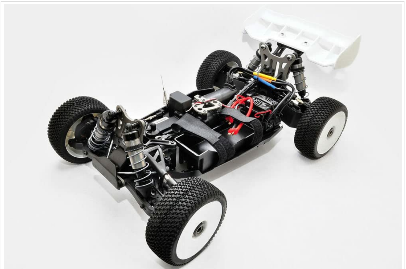
Figure 3.2: Top-down view of the Hyper VS chassis with the body removed, revealing the internal layout including the battery tray, ESC, motor, and servo.
