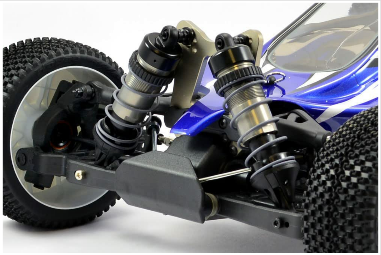
Figure 3.5: Close-up view of the front suspension system, including the shocks and control arms, designed for absorbing impacts.
