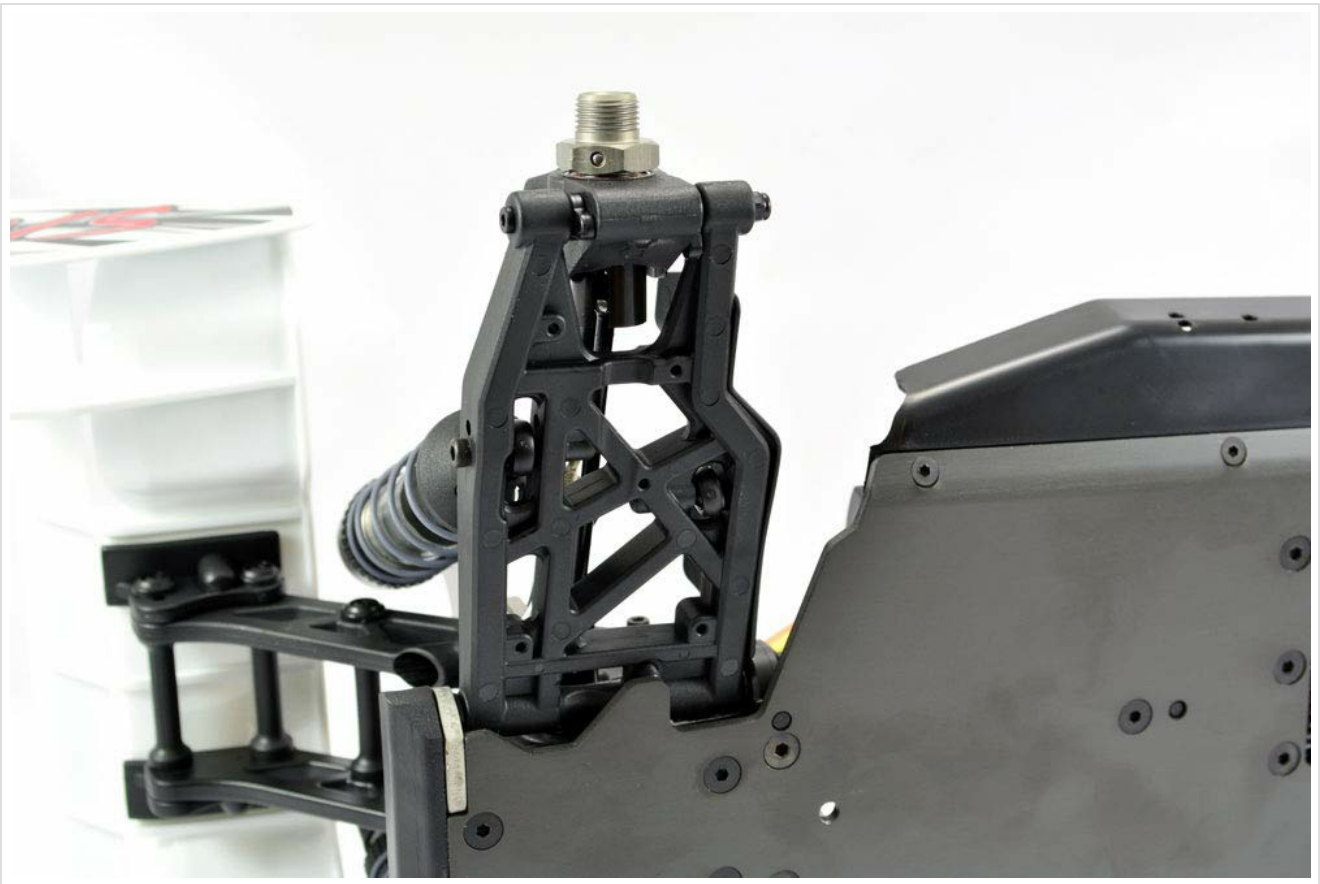
Figure 3.7: The robust front shock tower, a key component for structural integrity and suspension performance.
