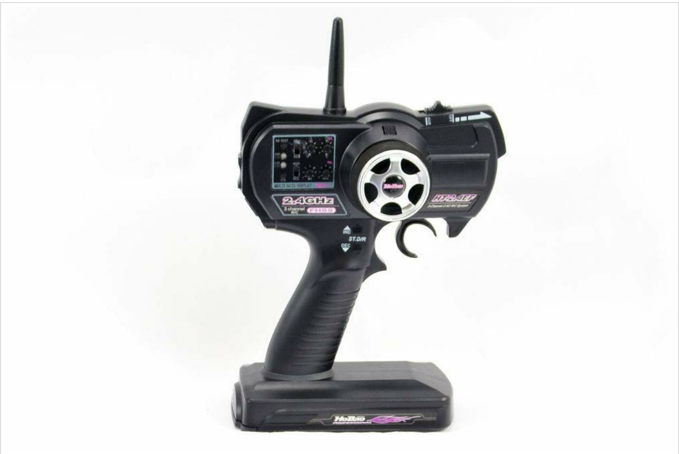
Figure 3.8: The 2.4GHz radio transmitter, providing precise control over the Hyper VS buggy.
