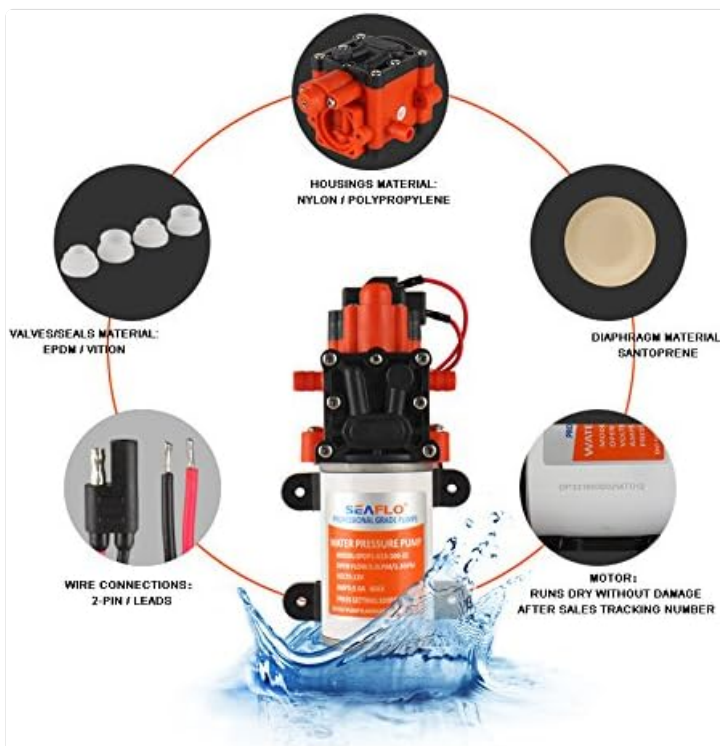
Figure 4: Diagram detailing the materials used for various pump components, including housings, valves/seals, diaphragm, and motor.
