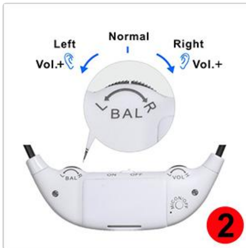
Figure 5: Headset controls for volume and left/right balance.
