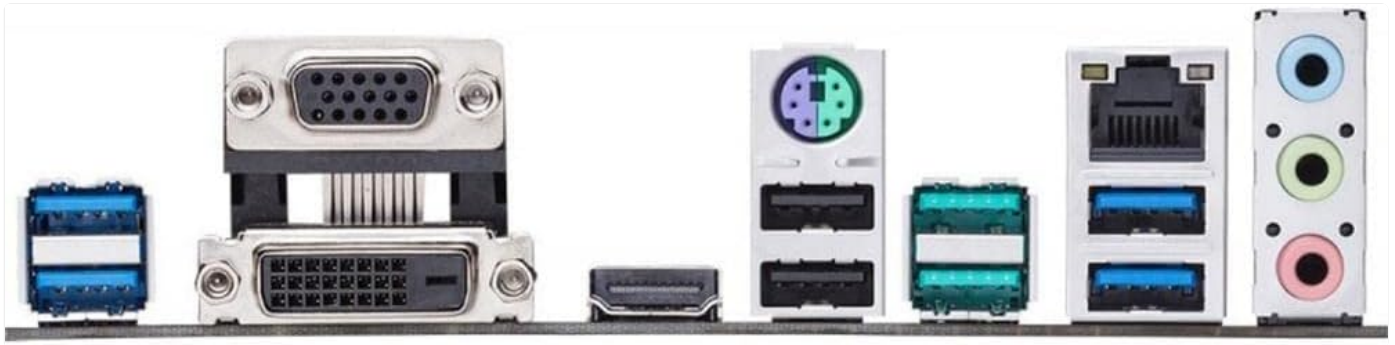
Figure 2.3: Detailed view of the rear I/O panel, including USB ports, video outputs (HDMI, DVI, VGA), LAN port, and audio jacks.
