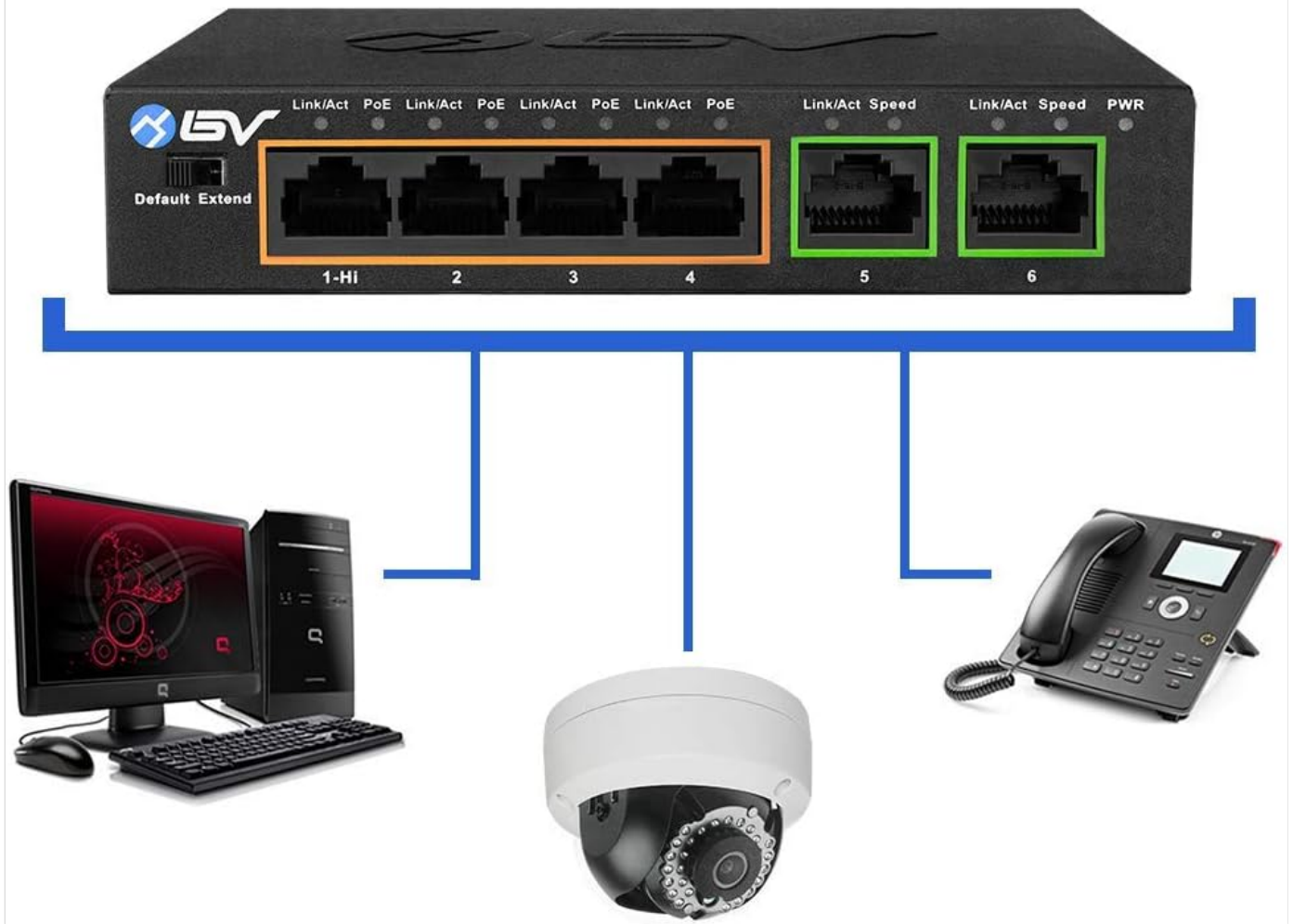
Figure 6: High Power capability of Port 1 (up to 60W).
