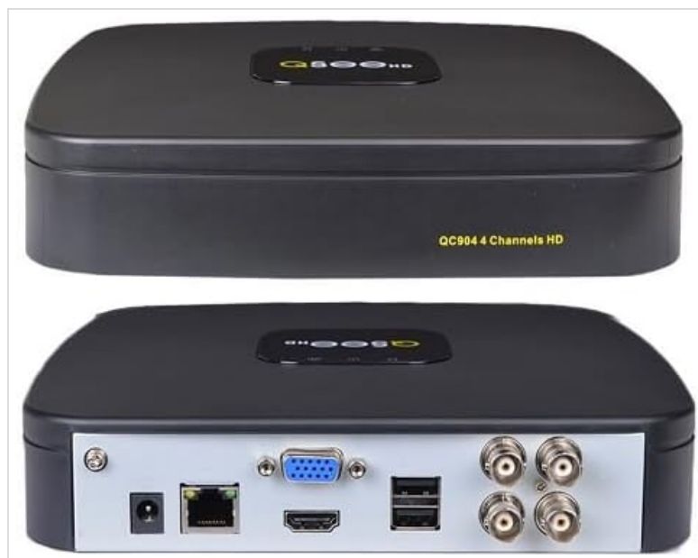
Image 3.1: Front and rear panel of the QC904 4-Channel DVR, showing connection ports.
