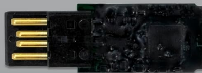
Epoxy resin sealed electronics (provides proof of tamper)
