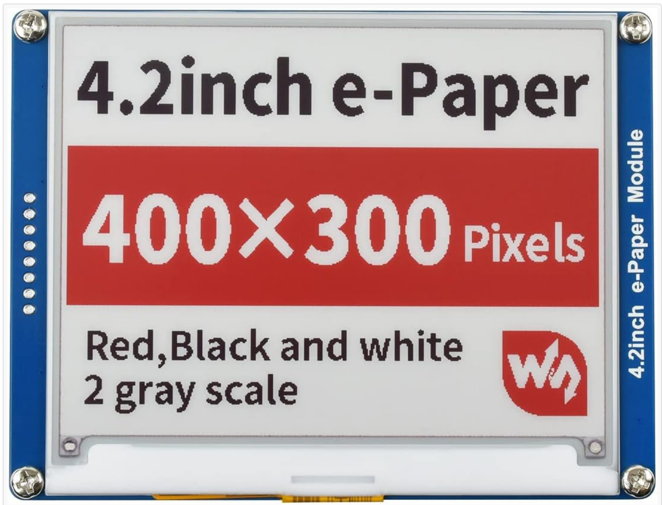
Figure 1: The Waveshare 4.2-inch E-Ink Display Module (B) displaying its specifications and capabilities in red, black, and white.
