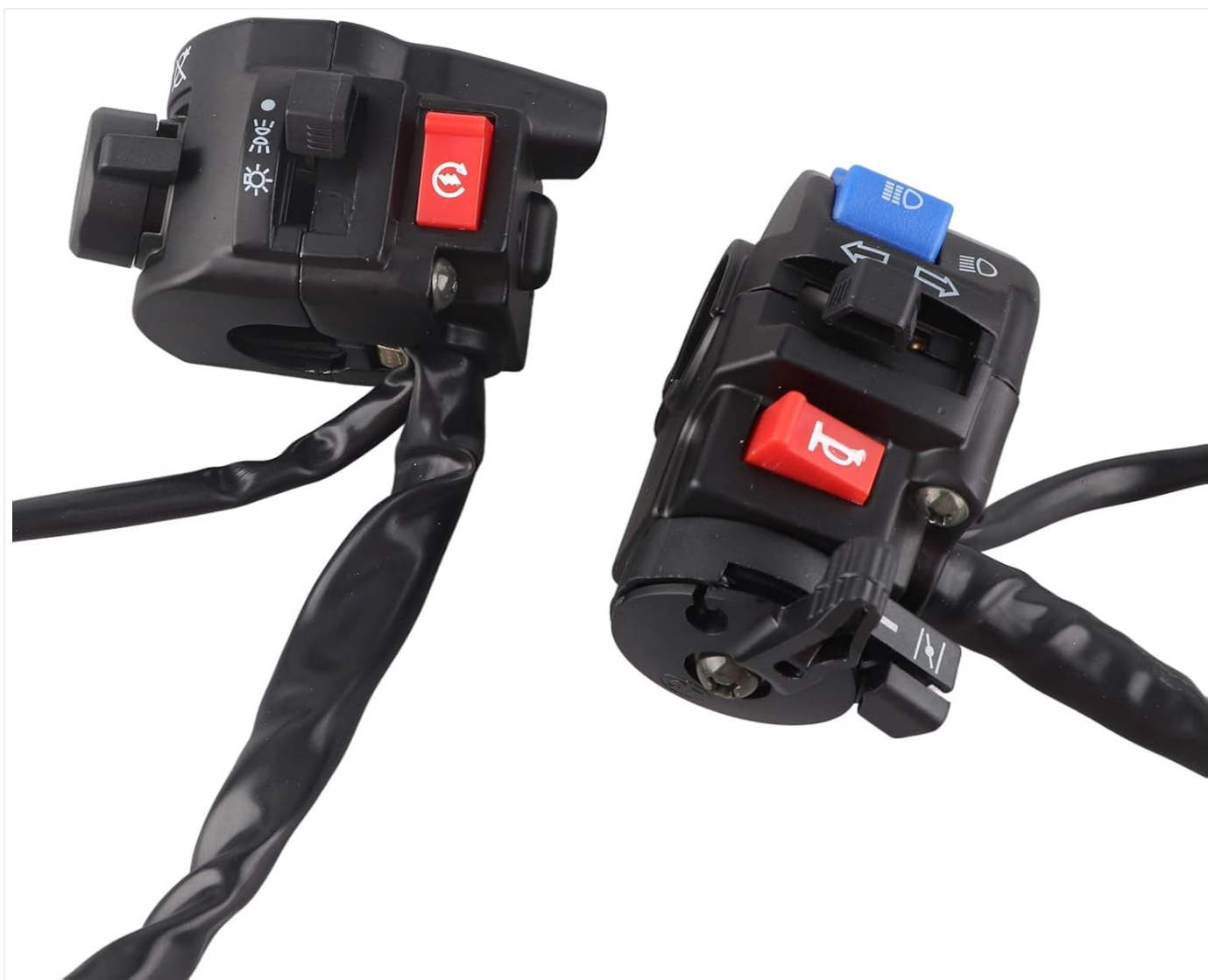
Image: A detailed view of the left handlebar switch, clearly showing the controls for turn signals, horn, and high/low beam headlights.
