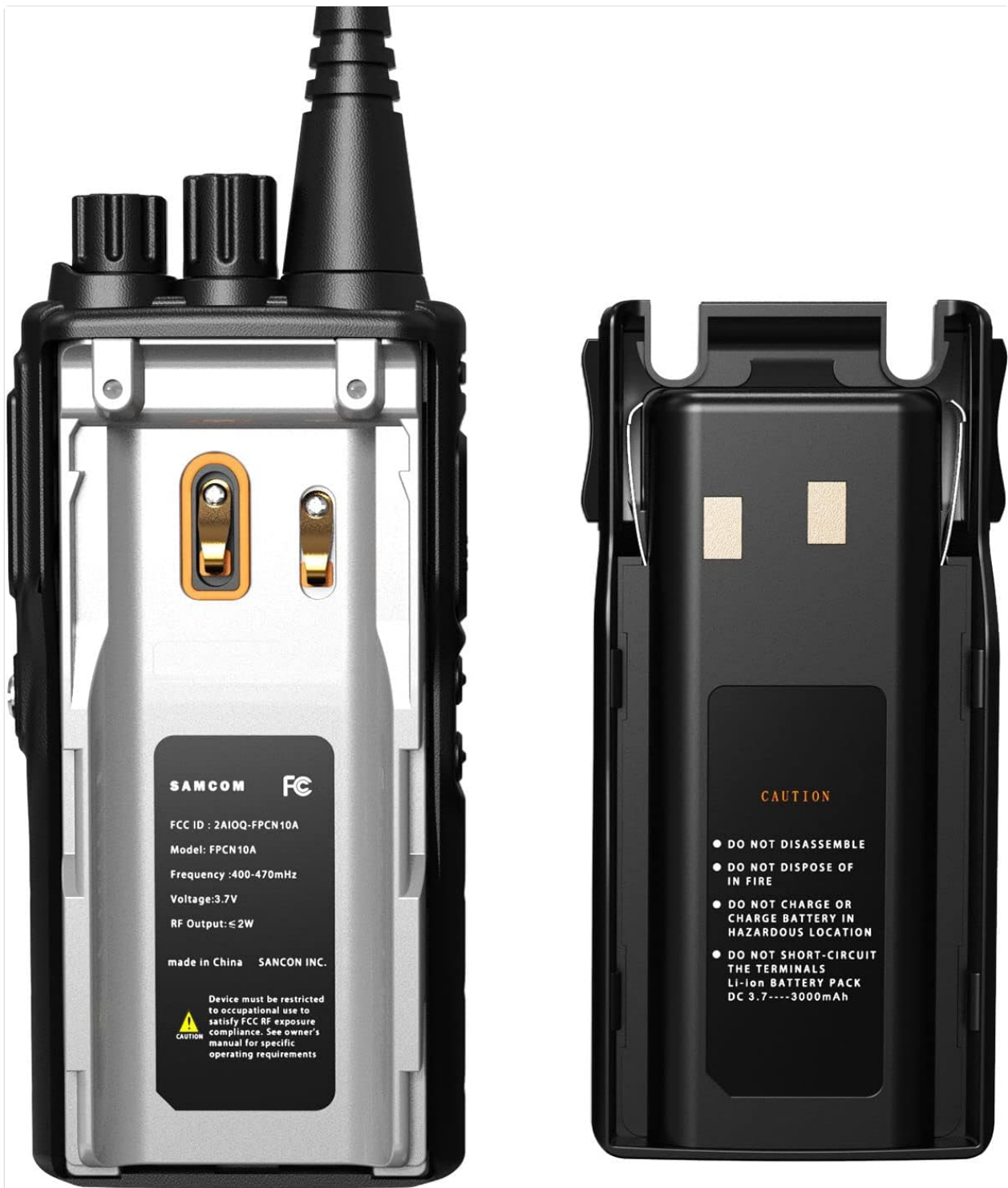
Figure 3: Rear View of Radio with Battery Removed. This image highlights the battery attachment mechanism and the FCC ID label on the radio's back.
