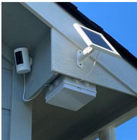
Figure 5: Outdoor Application Example (Solar Panel)
