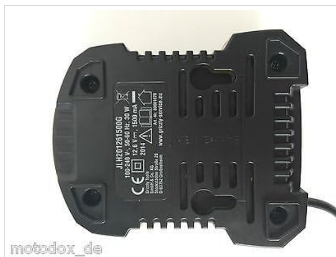
Figure 4: The underside of the charger, displaying the technical specifications label including model number, input/output details, and safety markings.
