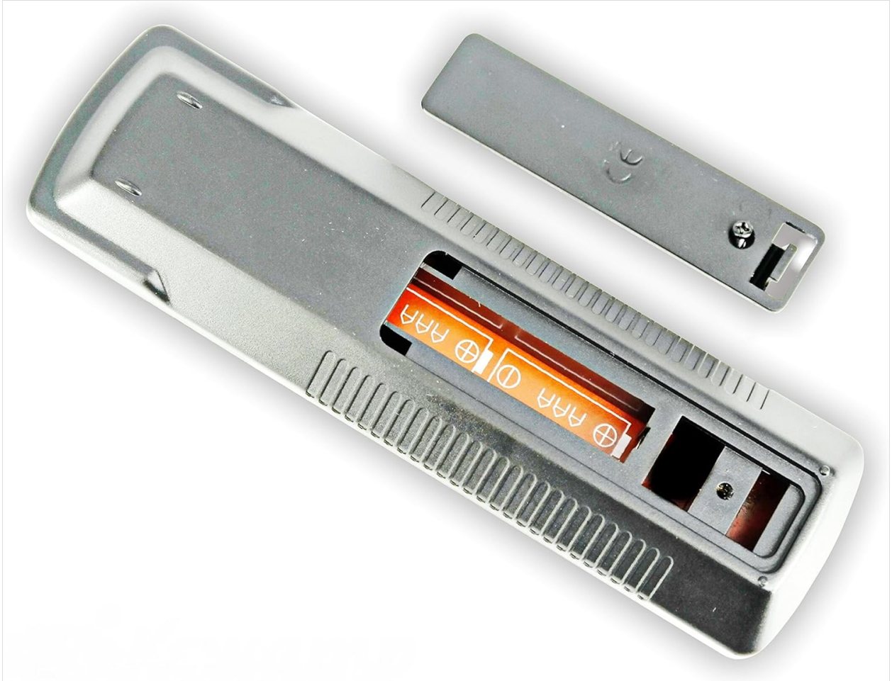
Image: The battery compartment of the remote control, open and ready for battery replacement. Ensure correct polarity when inserting new batteries.
