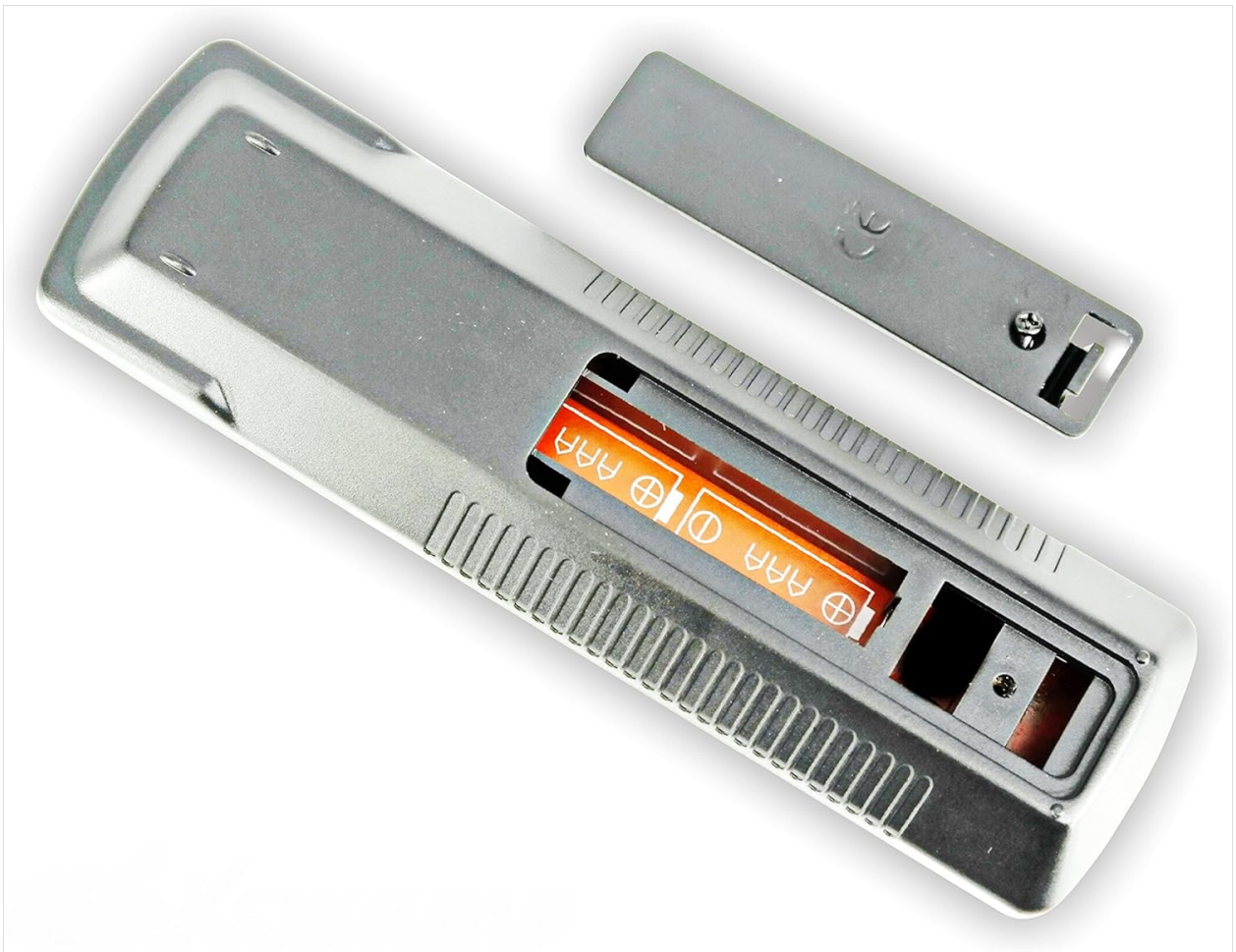
Image: The back of the Tekswamp remote control with the battery cover removed, revealing the slots for two AAA batteries. The correct orientation for battery insertion is indicated.
