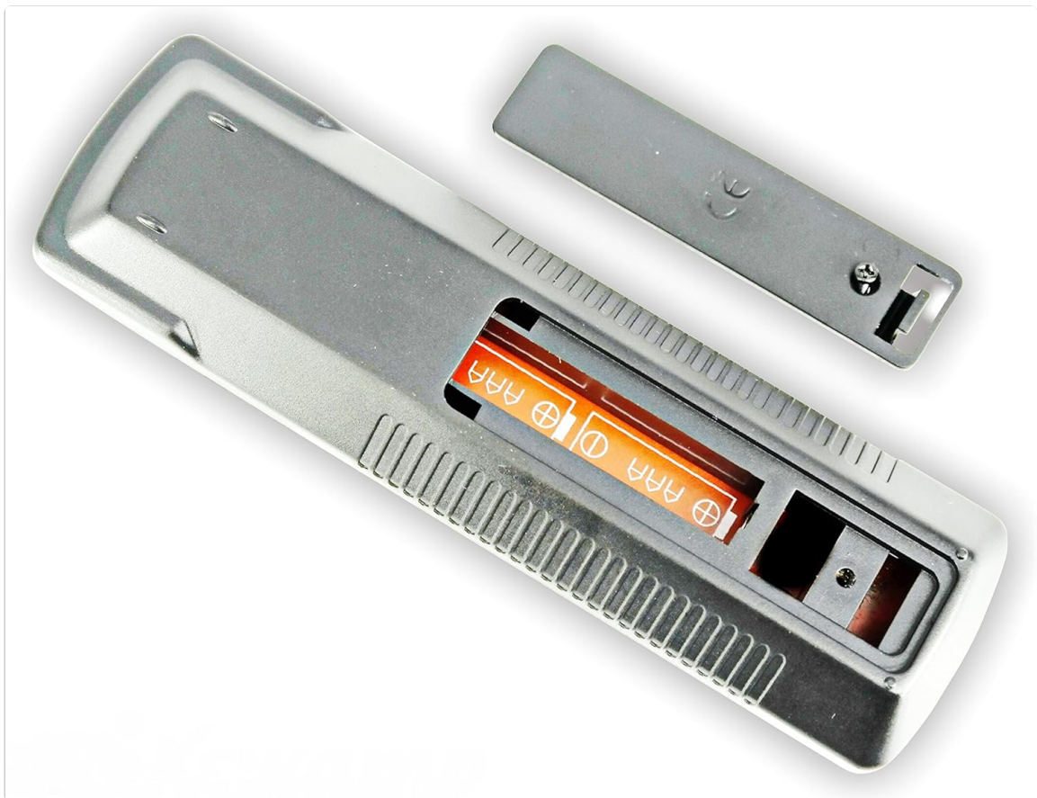
Figure 3: Open battery compartment, showing the correct orientation for AAA battery insertion.
