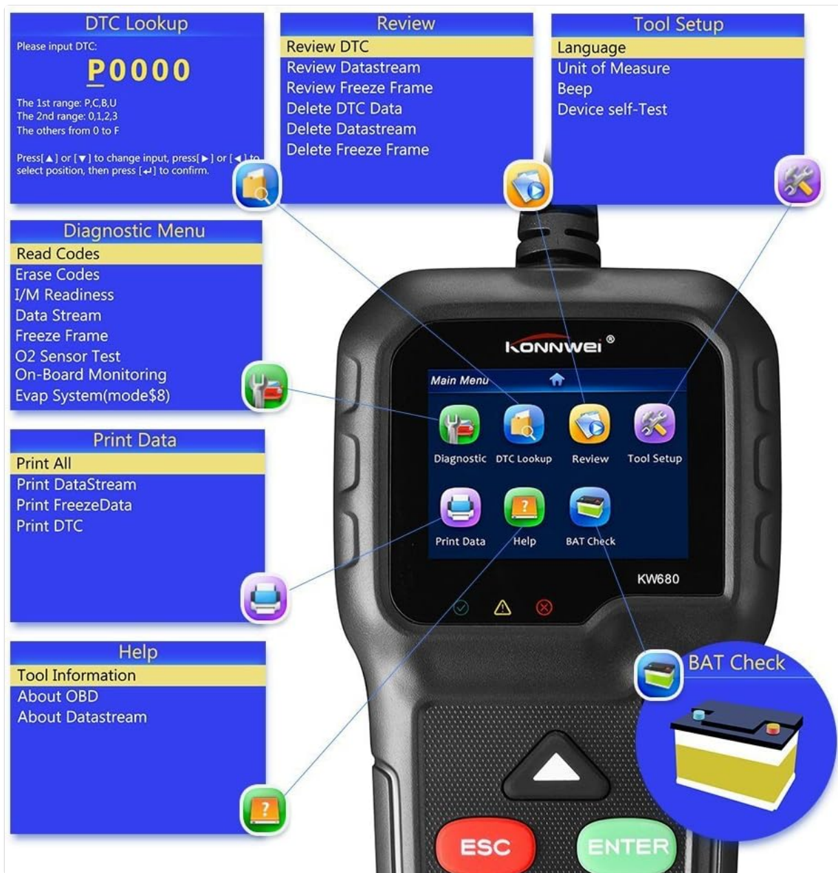
Figure 4.1: A detailed breakdown of the KW680's main menu and sub-menu options.
