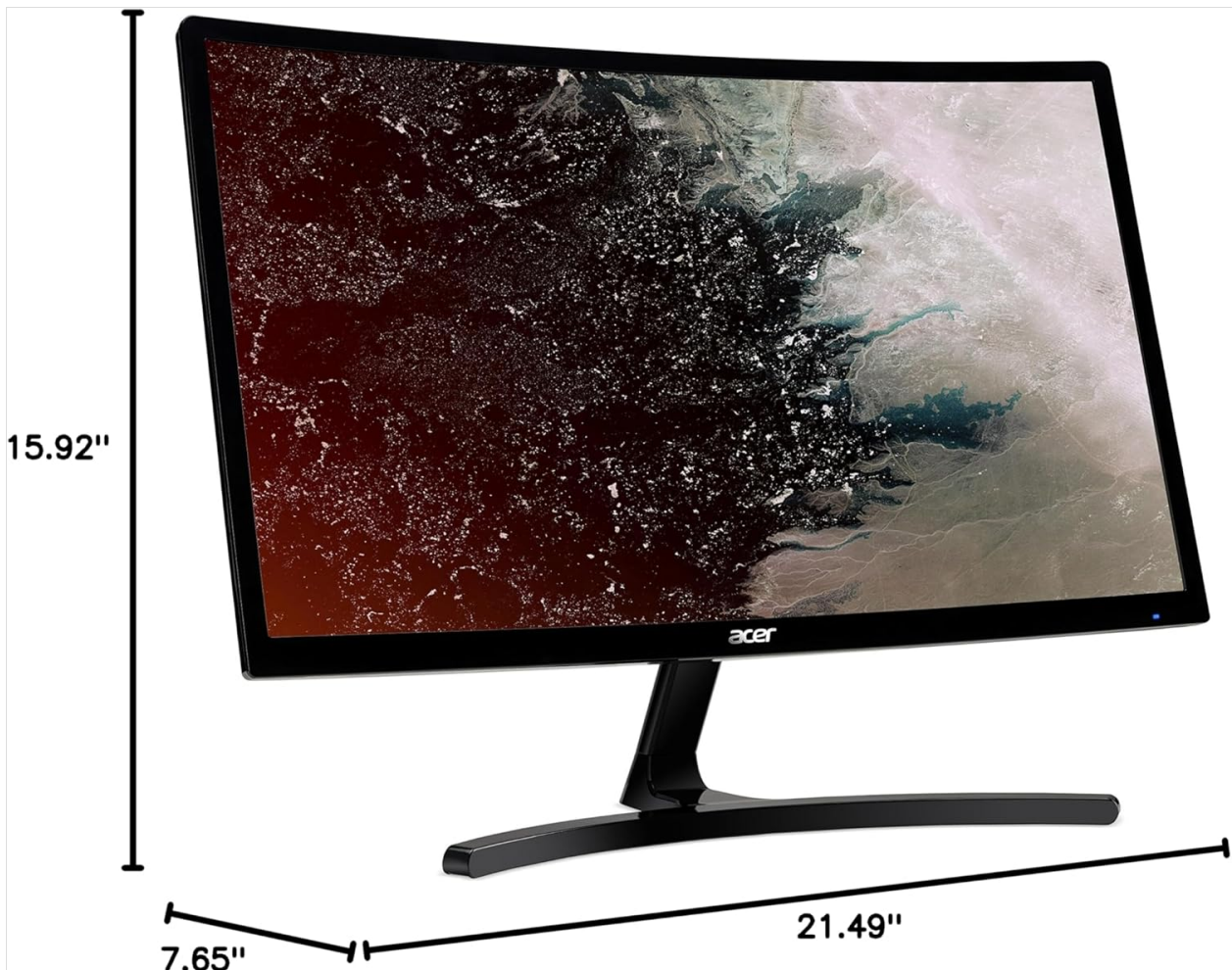
Figure 8.1: Physical dimensions of the Acer ED242QR Abidpx monitor, including width, depth, and height.
