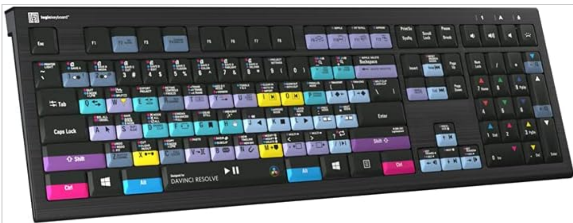
Image 3.1: A detailed top-down view of the keyboard, showing the various color-coded keys and their corresponding DaVinci Resolve functions and icons.
