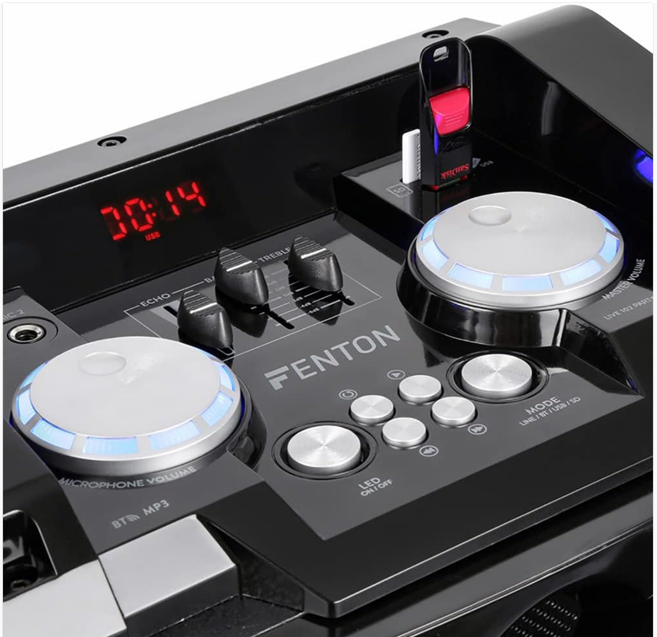
Detailed view of the top control panel, showing a USB flash drive inserted into the USB port, the SD card slot, and the media playback control buttons (Play/Pause, Stop, Previous, Next).
