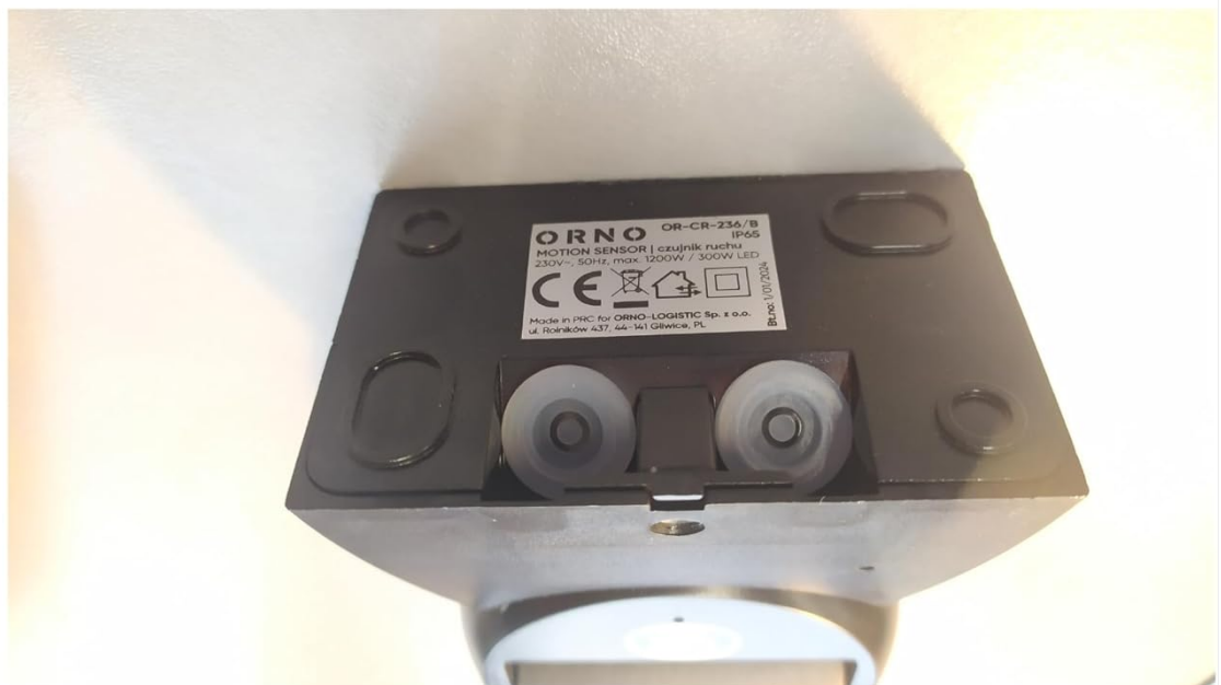
Figure 4.2: View of the sensor's base, highlighting the mounting points and sealed cable entry for secure installation.
