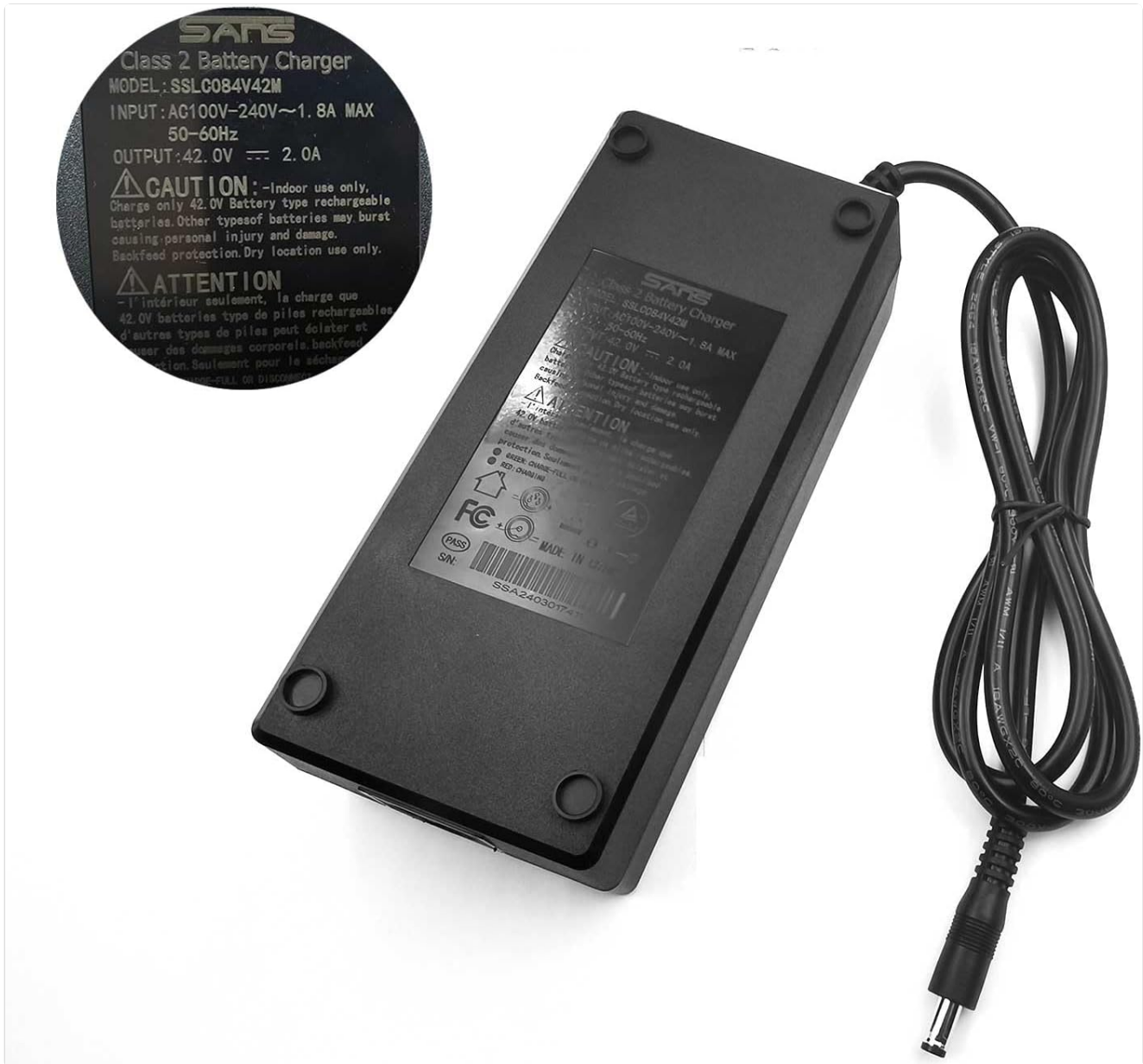
Figure 4: Bottom label of the SANS charger displaying detailed specifications and certifications.
