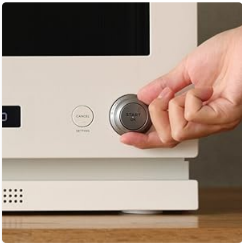
Figure 5: The right dial is used to confirm selections and start operation.
