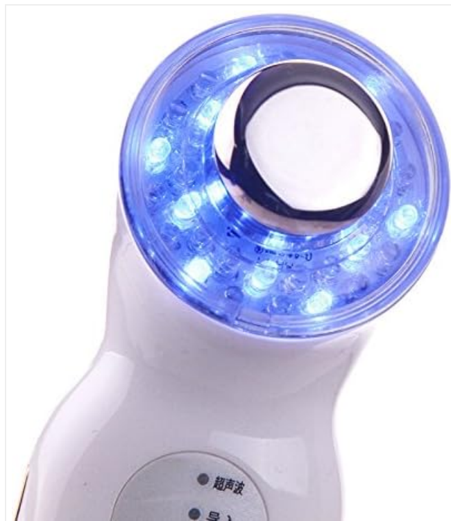
Figure 7.2: The device's treatment head illuminated with blue LED light, indicating the blue light therapy mode is active.
