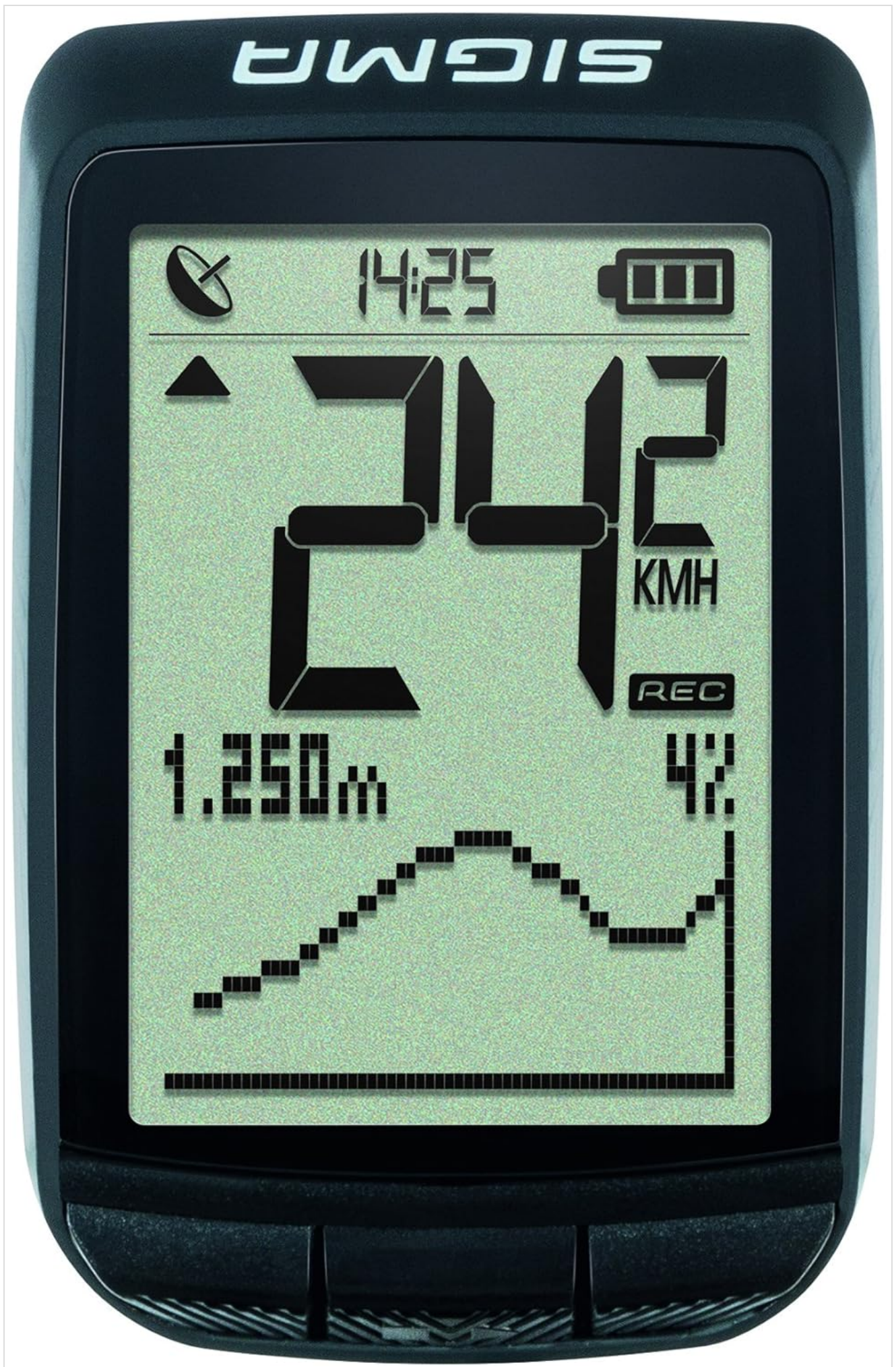
Figure 2.2: Front view of the Sigma Pure GPS Bicycle Computer showing current speed and a graphical altitude profile.
